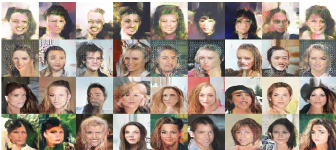
Figure 9.3: Samples generated by the DCGAN – First row: epoch 1 (FID = 137.11); Second row: epoch 8 (FID = 153.74); Third and fourth rows: epoch 13 (FID = 111.92).
